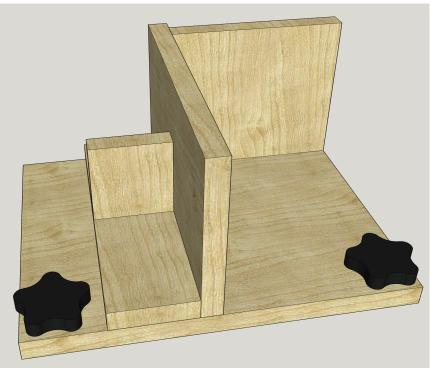
Very simple: Only 5 wooden parts. I have two T-Slot knobs to lock this jig down on my drill press table. Clamps will work just as well.
