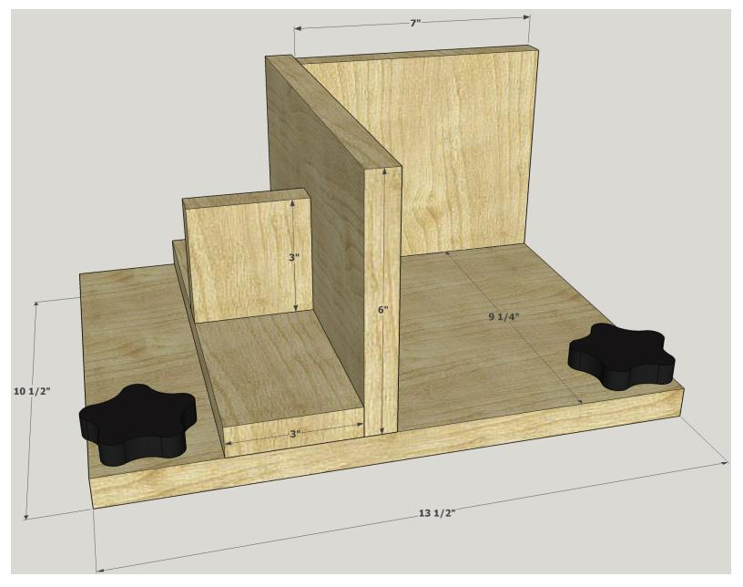
The location of my fence on my base was determined by my drill press. This may need to be changed to match your drill press. I made this so I could set my jig up flush with the front of my drill press table and the drill bit would be in the right place.
